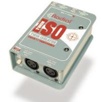
The Radial Twin-Iso is a balanced 2 channel, +4dB line-level isolator that has been specifically developed for professional touring systems as a means to eliminate hum and buzz caused by ground loops when interfacing various equipment such as two consoles, remote towers and drive racks.
