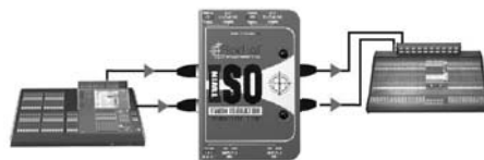
Using the Twin-Iso to isolate two mixers
