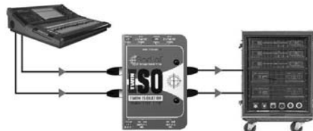
Using the Twin-Iso between mixer and amp racks
