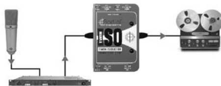
Using the Twin-Iso to eliminate noise
