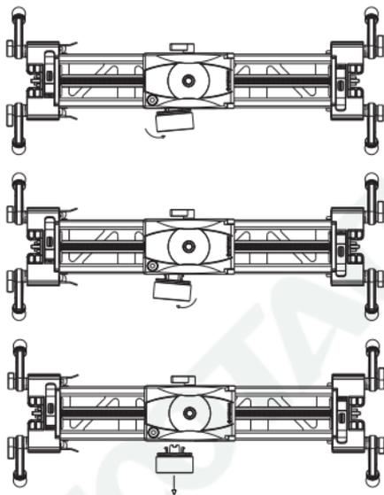
Firmly hold the flywheel and gently pull to the left, then do the same, but to the right followed by pulling the flywheel away from the carriage at 90 degrees. This will ensure safe removal of the flywheel from the carriage.
