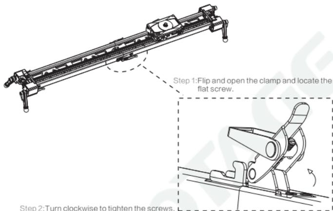
7. Use a suitable flat end screw driver to adjust tightness.
