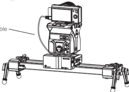
\* If using long lenses, please ensure the center of balance is adjusted properly prior to switching on. With its built-in sensor, the X2 Mini will automatically find its starting point after power up. If using the X2 Mini on a tripod, it will use the power up position as the starting point.
