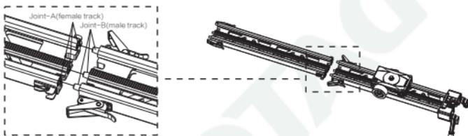
Step 3: Use the buckle locking system to lock the two tracks together. Check buckles are closed and tracks are secured together successfully prior to replacing and locking in place the foot stand.
