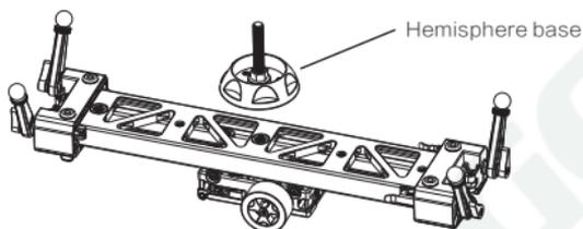
Step 2: Mount the hemisphere base on the tripod and adjust the slider until the carriage's spirit level shows the slider is horizontal, Lock into position.
