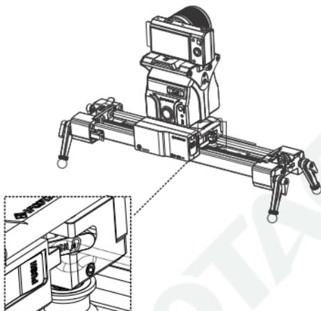
Step 3: Set up fully loaded slider at the angle you wish to use it and carefully test out counterweight. Increase or reduce weight accordingly. The pulley must be installed using an appropriate counterweight for the set up and weight of the camera and head.
