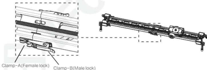
Step 4: Place the track connection plate on the underside of the joined track and secure with screws provided. Check that the plate is secure and is adequately supporting the track joint.
