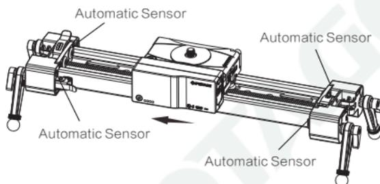
\*The carriage will stop automatically 10mm from the left foot stand.(The 1 axis slide module is equipped with a sensor which will move to the starting point and stop automatically)
