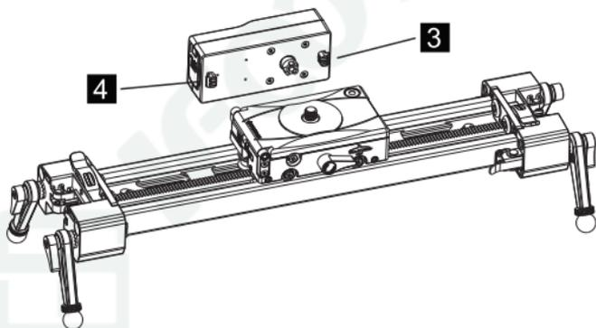
Step 3: Check that the single-axis module is securely attached to the carriage.
