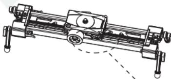
In order to prevent the carriage from moving, rotate the carriage locking control, following the direction of the arrow direction.
