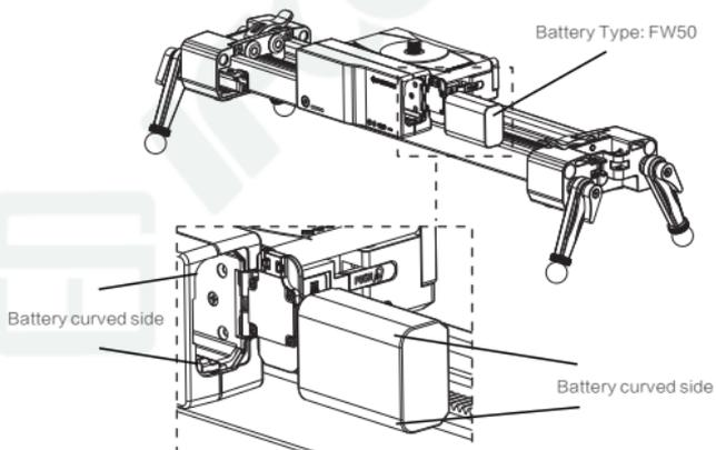
\*Insert the battery in the 1 - axis module, pay attention to the direction, DO NOT insert it in opposite direction.
