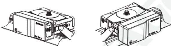
Step 2: Gently remove the single axis module from the carriage at a 90 degree angle to the carriage.
