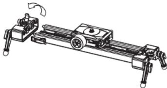
Step 2: Attach the track extension to existing track using the male and female connecting nodes. (see diagram).
