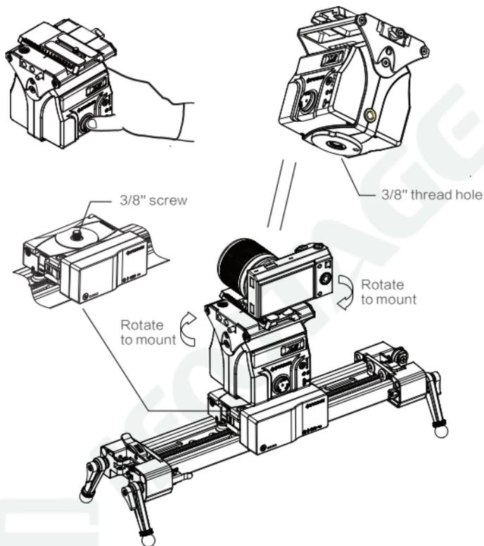
Step 1: Carefully place the thread 3/8" hole of the X2 Mini pan head onto the 3/8" screw on top of the Shark Slider carriage. Rotate clockwise.
