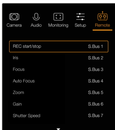
Remote-Einstellungen – Blackmagic Micro Studio Camera 4K
