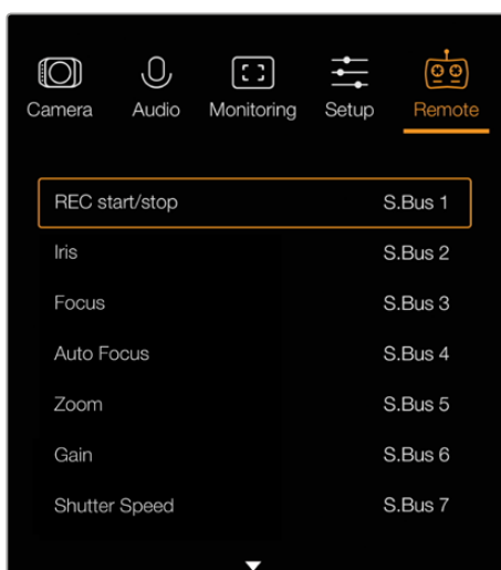
Настройки Remote на Blackmagic Micro Studio Camera 4K
