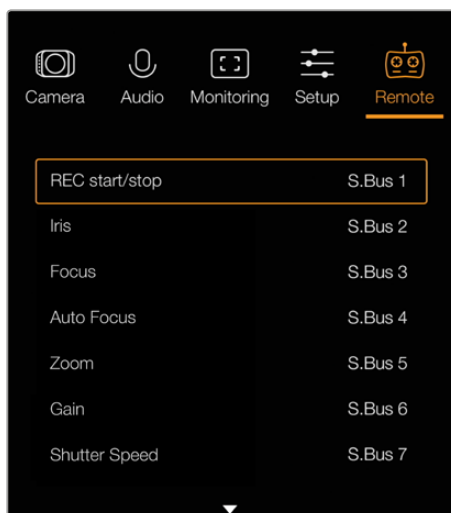
Remote settings – Blackmagic Micro Studio Camera 4K.
