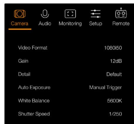
Camera-Einstellungen – Blackmagic Studio Camera Blackmagic Micro Studio Camera 4K
