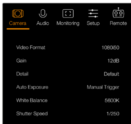
Настройки Camera на Blackmagic Micro Studio Camera 4K
