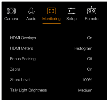
Monitoring settings - Blackmagic Micro Studio Camera 4K.
