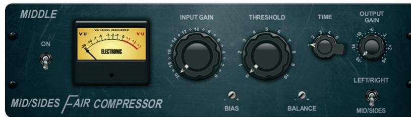
The Fairchild 670 tube compressor not only achieves record bids in high-end vintage gear auctions, it also delivers some of the finest colorations in compressor history. Two small trim VR's preset the control side chain action, a six-step switch determines the timing, and the two large Input and Threshold knobs adjust the levels. Our FAIR COMPRESSOR model is true to the original signal path, and conveniently provides models for dual, stereo-linked or M/S operation. (Inspired by Fairchild 670\*)
